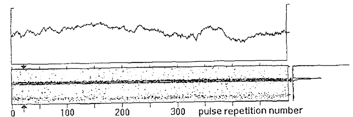
Figure 3 - Simulated chimney reflections fluctuating due to wind
