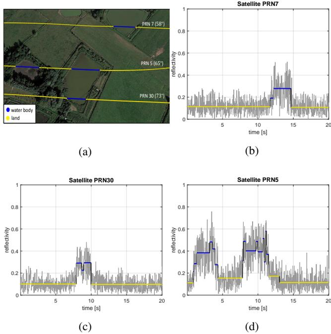
FIGURE 4 – Detection of in-land water body surfaces using the proposed automatic radar signal segmentation technique.
