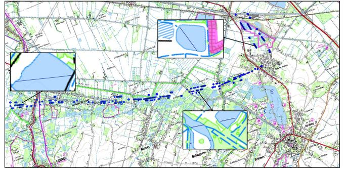
FIGURE 3 – The detected water body surfaces using our proposed radar technique for three satellites in study.
