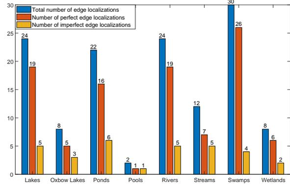
FIGURE 5 – Statistics of water body edge localization by the proposed radar technique per water body type.
