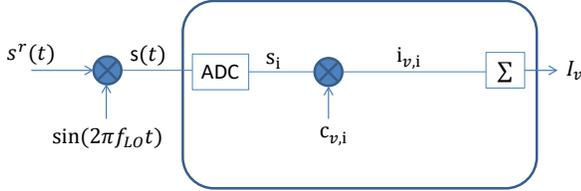
FIGURE 1 – Radio frequency GNSS receiver block diagram
