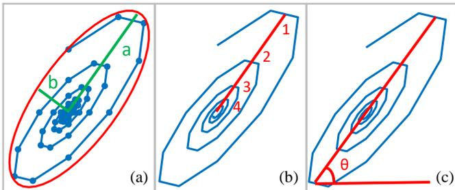
Figure 2. Phase diagram dispersion (a), the number of spirals (b) and orientation (c)
