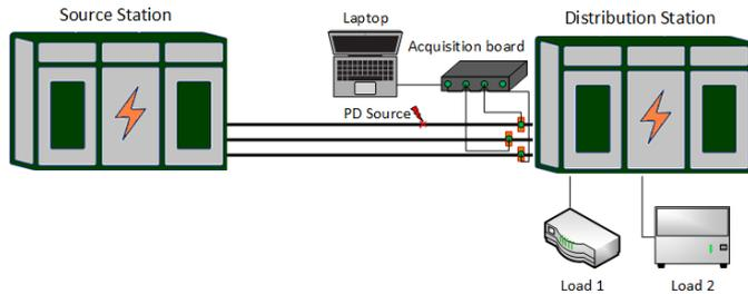
Figure 3. The power distribution network benchmark
