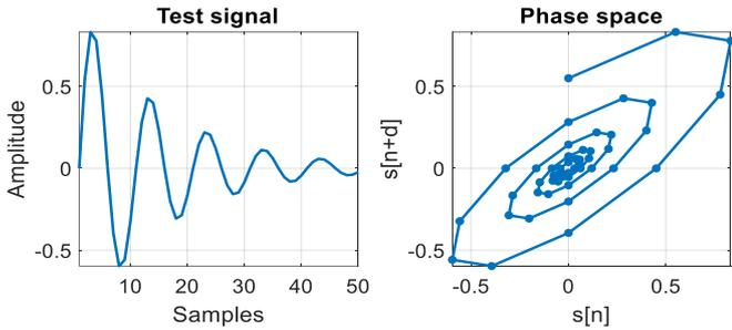
Figure 1. The test signal and its phase diagram representation
