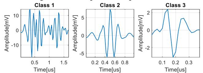
Figure 6. The three classes of transient signals
