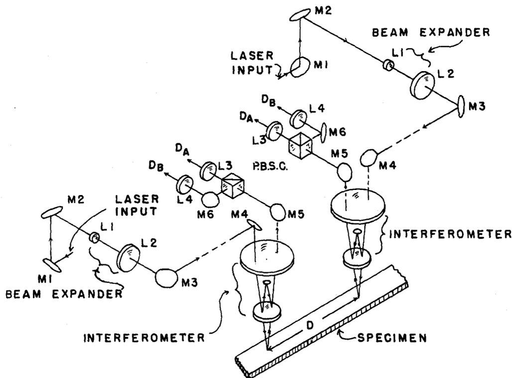
Fig. 2. — Dual laser interferometer (Fizeau).
