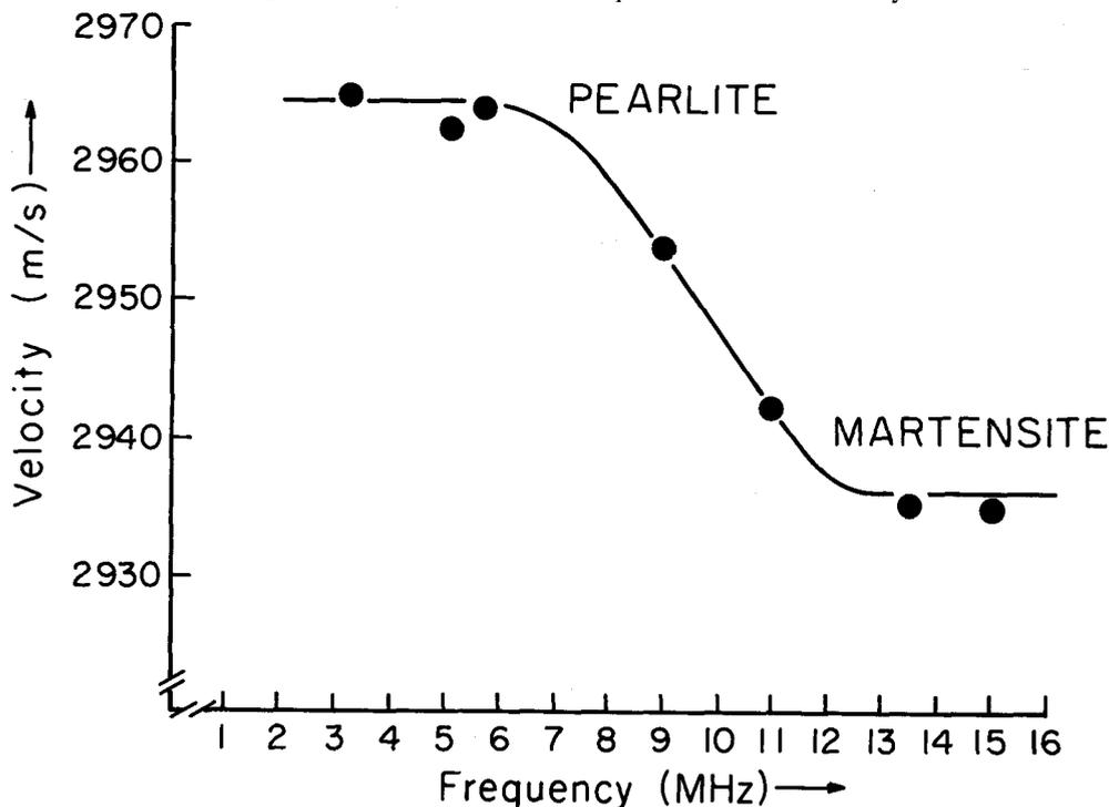
Fig. 6. — Variation of the apparent Rayleigh wave velocity with frequency (reciprocal of depth of penetration) in AISI 1045 steel. Regions of constant velocity (e. g., martensite) occur when the Rayleigh waves probe uniform layers of material.
