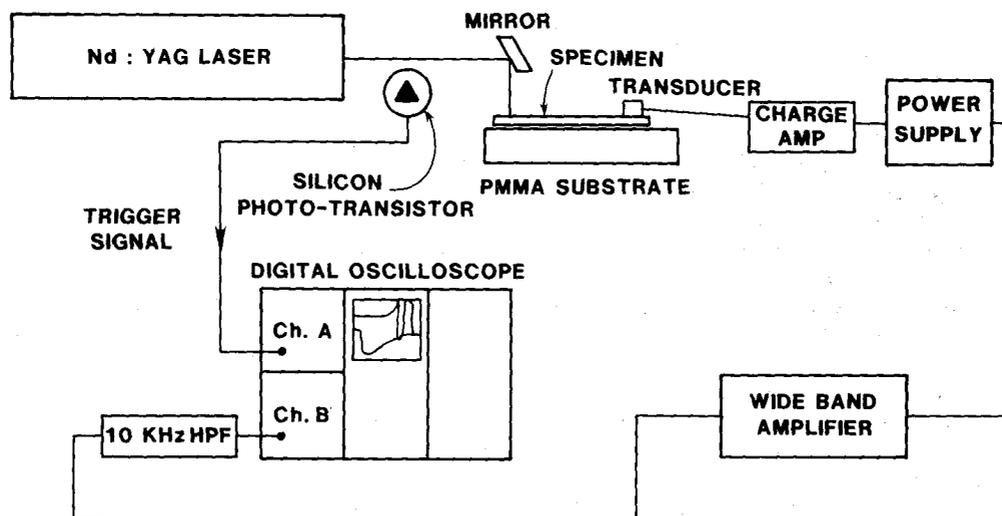
Fig. 1. — Sound velocity measurement system based on laser generation and piezoelectric detection of the propagating sound waves.
