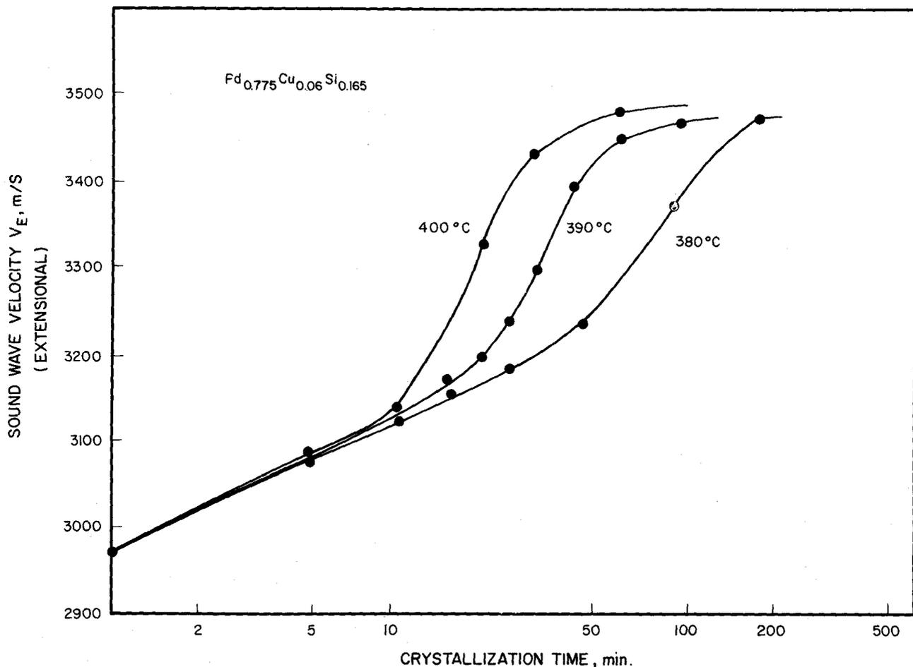
Fig. 3. — Variation of extensional wave velocity in PdCuSi during transition from amorphous to crystalline state as a function of crystallization time.
