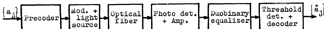
Fig. 1 Block diagram of an optical fiber communication system applying duobinary equalizer in the receiver.
